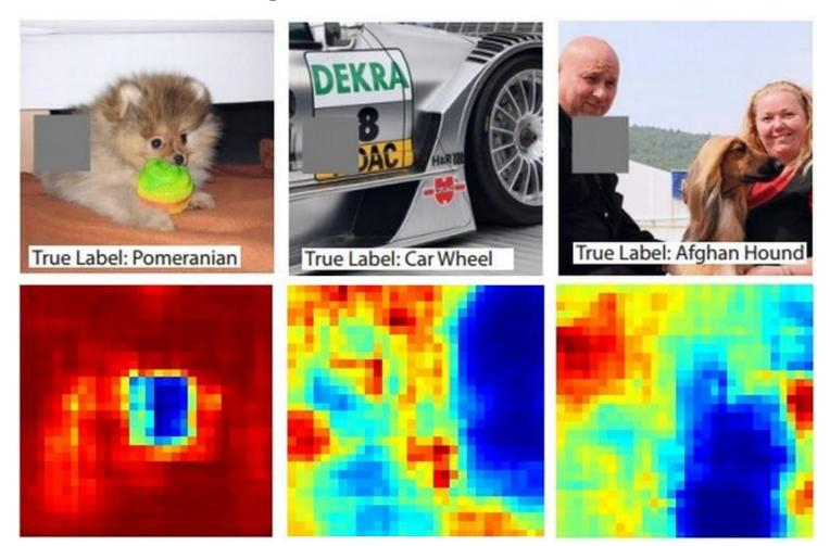
Figure 9: By constructing a heatmap of classification accuracy when a certain part of the image is occluded, we can identify the most important parts of the image for classification (blue)
