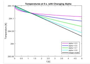
We initially observe a period of "super-diffusivity" until around 1.3s, in which the lower values of  $\alpha$  result in a higher rate of diffusion.
